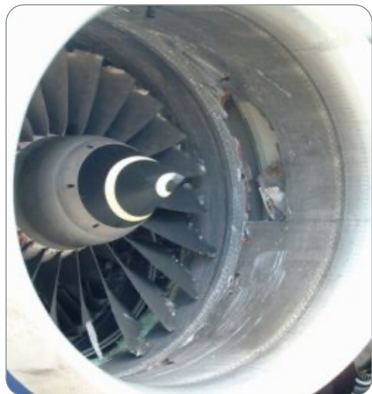
Figure 4. Fan Blade off causing damage
