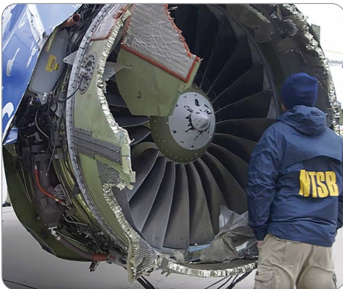
Figure 4. Fan Blade off causing damage
