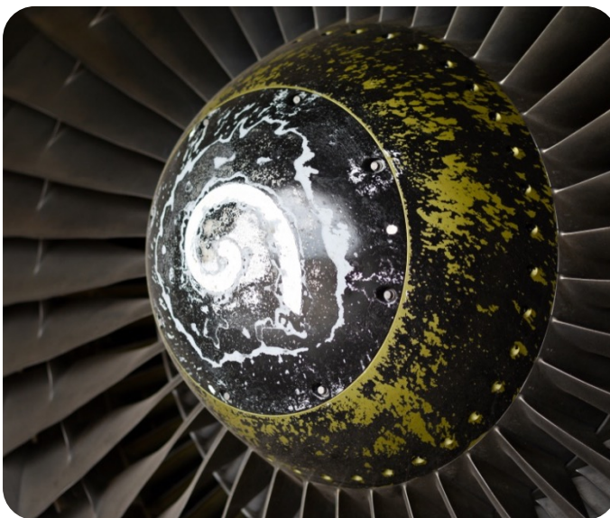
Figure 3. Partially damaged spinner cone (left) and fan blade (right) due to Bird hit
