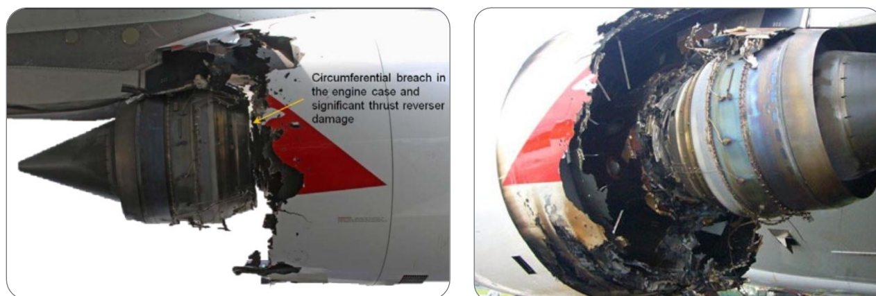
Figure 5. Uncontained blade out event caused severe disruption to engine in mid-air
