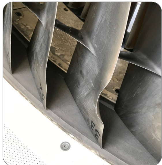
Figure 3. Partially damaged spinner cone (left) and fan blade (right) due to Bird hit
