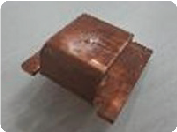
Figure-4: Small and rugged antenna element
